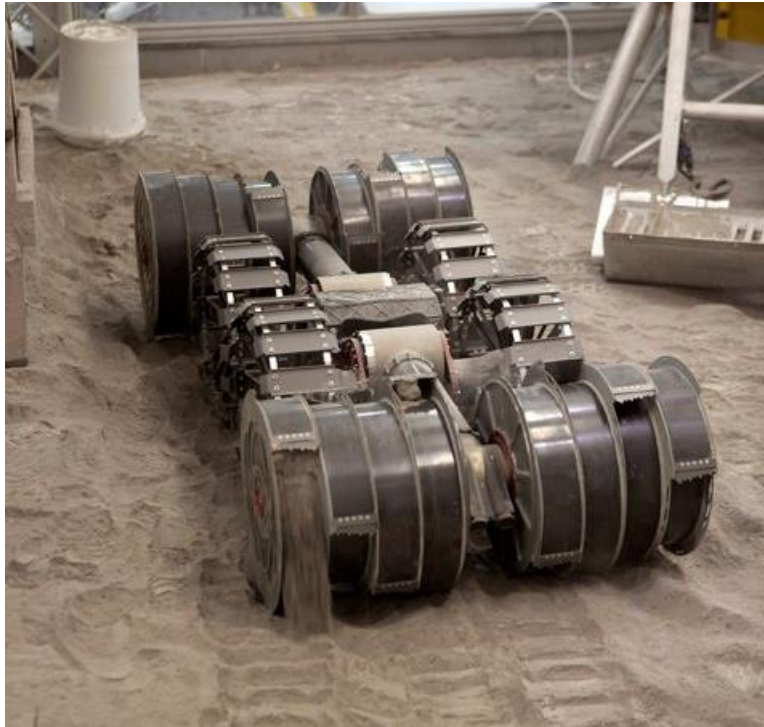
Figure 45. RASSOR 2.0 Unloading Simulated Regolith
